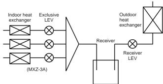
\*In COOL mode, the two indoor coil thermistor (one main and one sub) sense temperature ununiformity (super heat) at the heat exchanger, and when temperature difference have developed, the indoor coil thermistors adjust LEV opening to diminish the super heat. This action is called Evaporation Temperature Protection.
